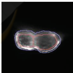
Figure 4: The Watershed segmentation (outline line) and the first rough identification of the chambers (inside line).
