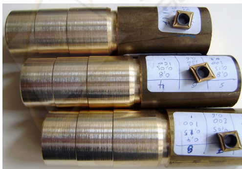
Figure 2: Machined specimens and inserts.
