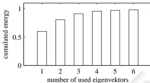
Figure 5: Cumulated energy using different numbers of KLT coefficients.
