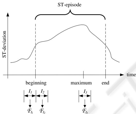
Figure 1: Intervals used to extract features. Although exact timing and number of the intervals may vary, the outlined timing (just before and after the annotated starting point ( $I_1$  and  $I_2$ , respectively) and around the maximum ST-deviation ( $I_3$ ) of the transient ST-episode) is common.
