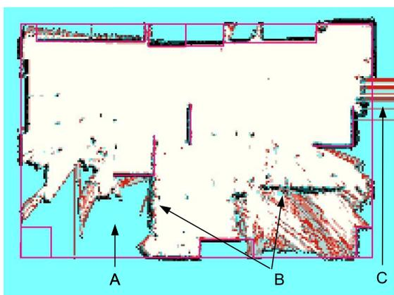
Figure 4: Map built by laser range finder readings at the end of the experimental test in an indoor environment. The black lines represent real obstacles.
