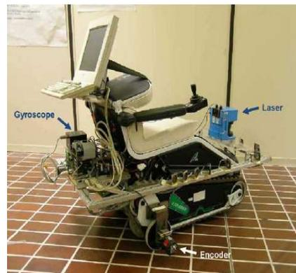
Figure 2: TGR-Explorer with data acquisition system.
