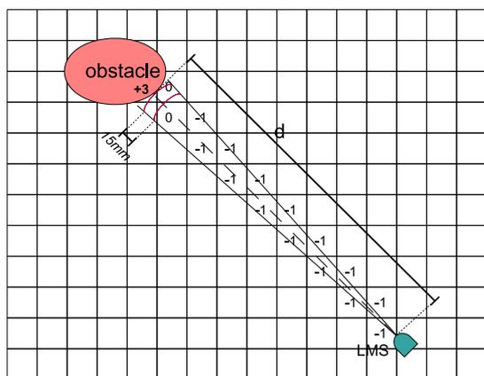
Figure 3: Histogramic Grid Update using a Laser Measurement System (LMS).
