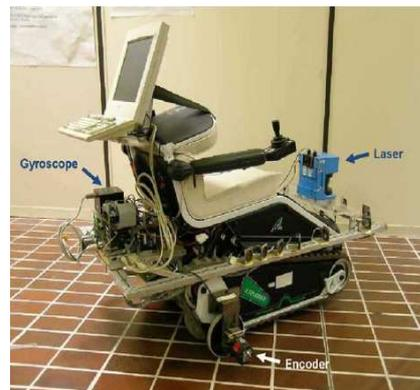
Figure 2: TGR-Explorer with data acquisition system.
