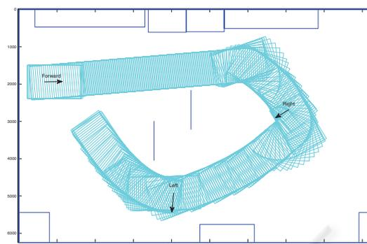
Figure 5: Simulation test in an environment crowded with obstacles. The path performed by the wheelchair with the second level of autonomy is depicted (clockwise direction of motion). The arrows represent the directions chosen by the user in the corresponding instant. The (blue) straight lines reproduce the obstacles. The values are in millimeters.
