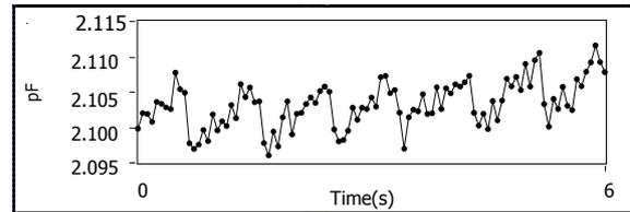
Figure 4: Capacitance measurement for electrodes mounted on the wrist.
