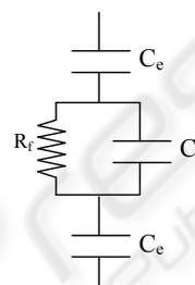
Figure 2: Electrical model for finger impedance.
