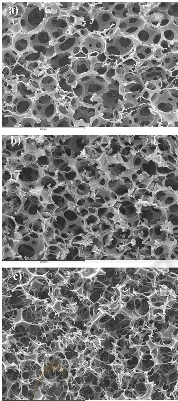
Figure 1: Scanning electron microscopy pictures of cross-sections of PEA scaffolds cross-linked with 5% (a), 10% (b) or 20 wt % (c) of TrEGDMA (see text).
