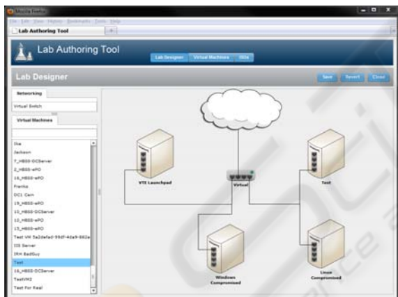
Figure 4: Virtual lab network configuration interface. Authors select virtual machines and network components by name from the left-hand panel and drag them into the lab configuration. Lines are dragged between components to create a network connection.
