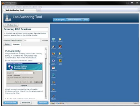
Figure 6: Authoring interface with active connection to the desktop of a virtual machine. On the left is the task panel, showing the task the author is currently completing.
