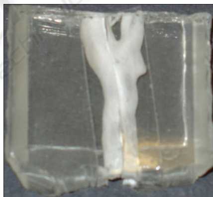
Figure 7: PDMS carotid channel by means of a TDP technique.
