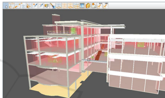
Figure 6: A structural view of a building. This view is required for structure engineers. The corresponding graph provides all elements needed to make structure calculations.
