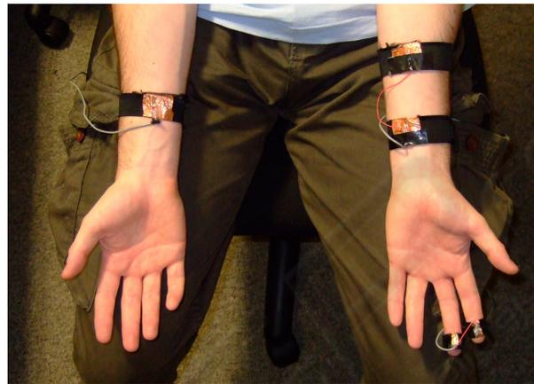
Fig. 1. ECG (HRV) and GSR sensors used audience biosignals recording.
