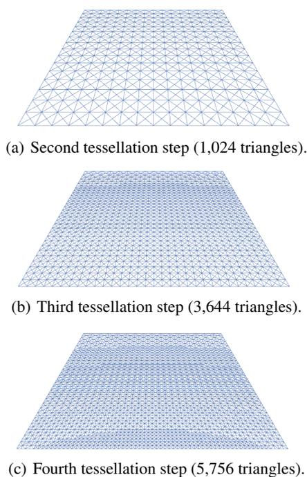
Figure 3: Sample tessellation using a distance criterion.
