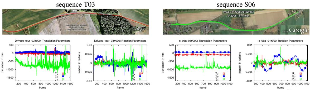
Figure 4: Top: The road on which our system was tested (from Google Earth) Bottom: Estimated vehicle egomotion: the estimated translation  $T = (T_x, T_y, T_z)$ , and the rotation provided as  $R = \alpha \mathbf{a}$ , where  $\alpha$  is the rotation angle and  $\mathbf{a}$  the axis.
