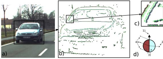
Figure 3: Illustration of the feature extraction level: a) one image; b) the 2D-primitives extracted; c) a detail of b); d) symbolic representation of a 2D-primitives, with 1-orientation, 2-phase, 3-colour, and 4-optical flow.
