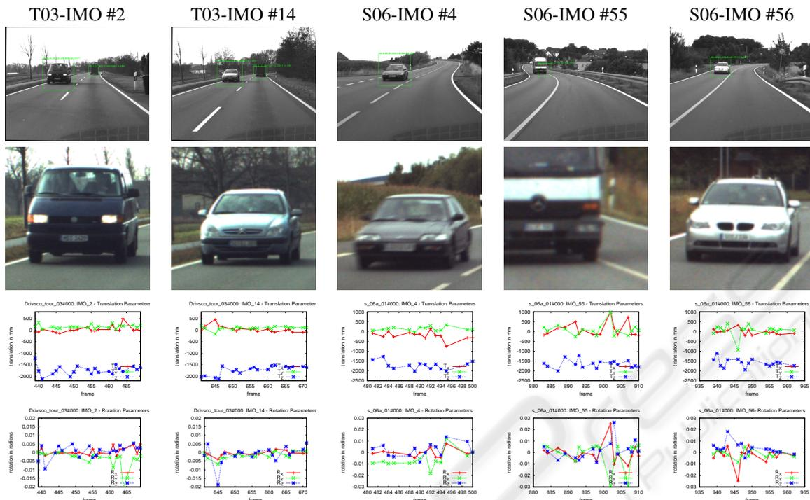
Figure 7: Example IMOs, two of which were taken from the sequence T03, and three from the sequence S06. The first row shows the detected IMOs; the second the high resolution ROI; the third the estimated translation, provided as  $T = (T_x, T_y, T_z)$ ; and the fourth the estimated rotation, provided as  $R = \alpha \mathbf{a}$ , where  $\alpha$  is the rotation angle and  $\mathbf{a}$  the axis.
