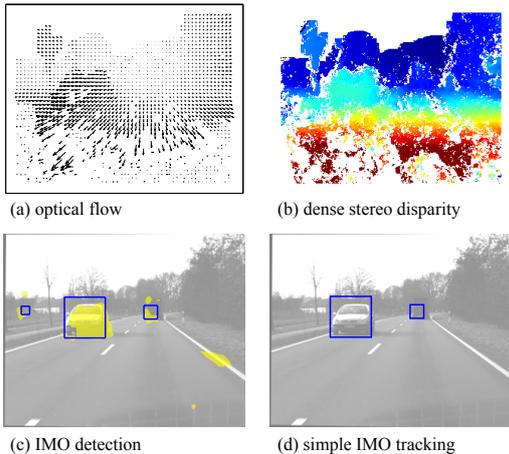
Figure 2: Illustration of the IMO detection level: a) the optical flow; b) the dense disparity; c) the low-level independent motion measure (yellow) and the detected IMOs after world-knowledge integration (blue boxes); d) the IMOs remaining after the simple tracking stage.
