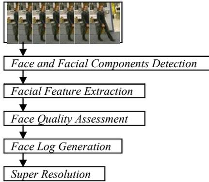
Figure 1: Block diagram of the proposed system.
