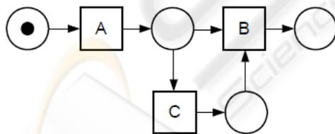
Figure 4: Petri Net of the SAP Transaction *Create Order*.
