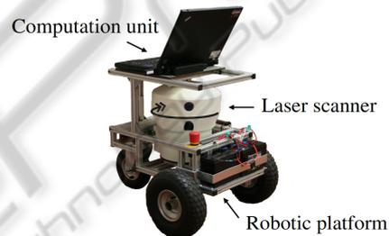
Figure 1: Hardware set-up.
