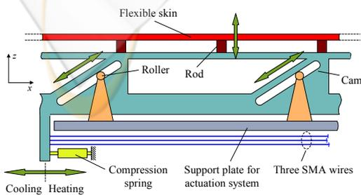
Figure 1: The actuation mechanism concept.
