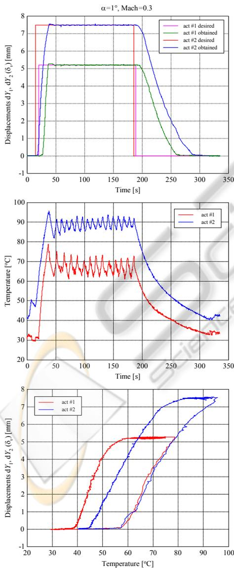
Figure 6: Bench test for  $\alpha=1^\circ$ ,  $M=0.3$  flight condition.
