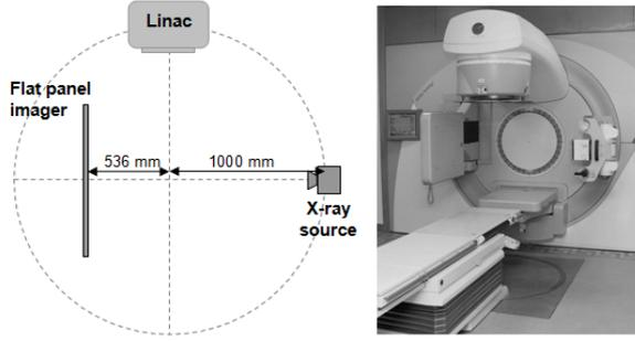
Figure 1: Medical linear accelerator with integrated X-ray cone-beam CT system.
