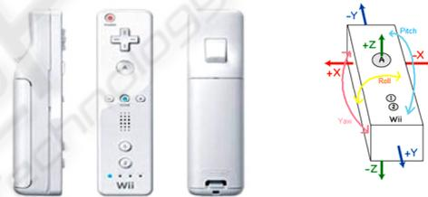
Figure 1: Wiimote and its accelerometer axes.
