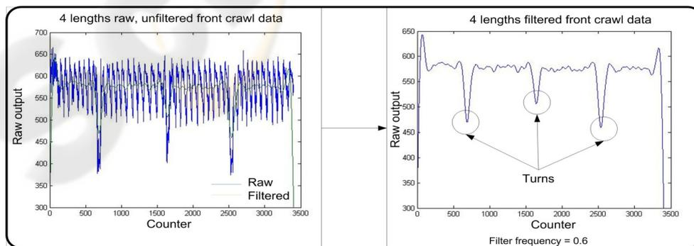
Figure 3: Butterworth filter on 4 lengths of front crawl data.
