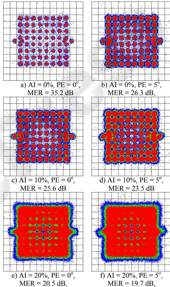
Figure 7: I/Q constellation of the DVB-T with 64-QAM, 8k mode and in case of *AI* and *PE* presence (DVB-T channel correction and all pilots ON).
