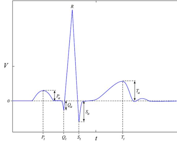
**Fig. 1.** Example of four latency times (features) measured from the P, QRS and T complexes of an ECG heartbeat for fiducial-based feature extraction.
