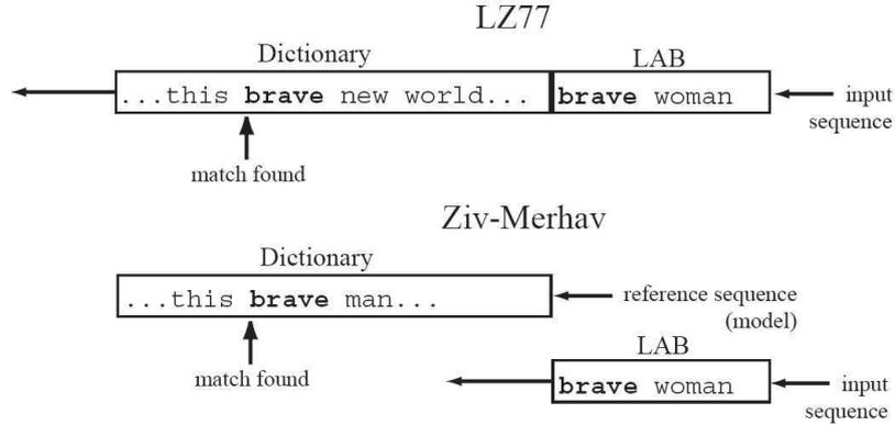
**Fig. 2.** The original LZ77 algorithm uses a sliding window over the input sequence to update the dictionary; in our implementation of ZM cross parsing algorithm, the dictionary is static and only the lookahead buffer (LAB) slides over the input sequence.
