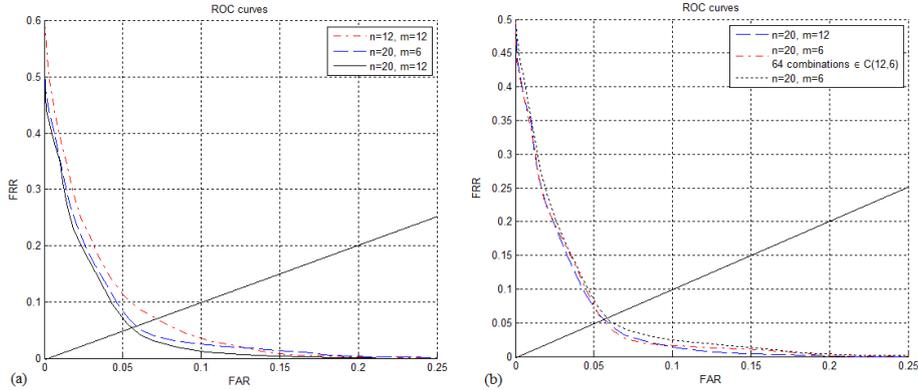
**Fig. 5.** ROC curves for the verification task (the solid straight line has slope 1, for reference purposes). Left plot: results for different  $n$  and  $m$  values; notice the improvement with the increase of  $m$  and  $n$ . The best equal error rate (EER) is close to 6%. Right plot: results for single classifiers versus a bank of 64 classifiers with the same structure for combination of multiple source acquisition signals.
