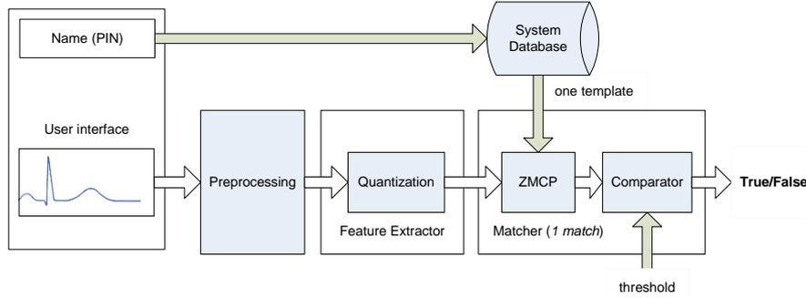
**Fig. 3.** Block diagram of the implemented system, for the authentication task, is shown using the five main modules of a biometric system, i.e., sensor, preprocessing, feature extraction, matcher and system database.
