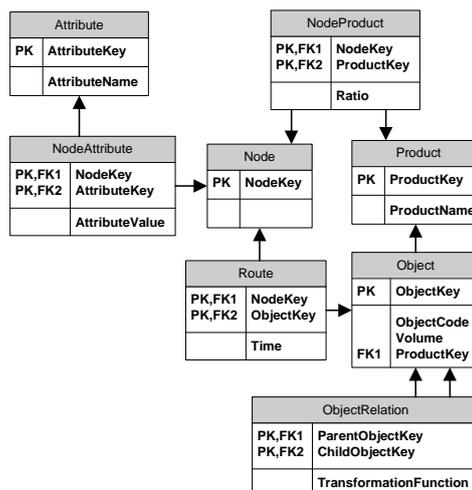
Figure 3: Database schema for the traceability graph.
