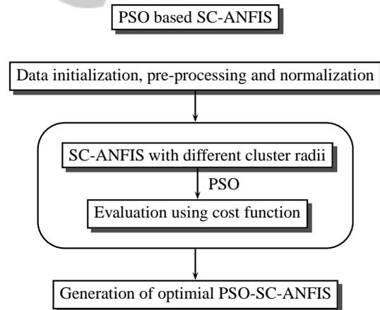
Figure 4: Flowchart for hybrid PSO-SC-ANFIS scheme.
