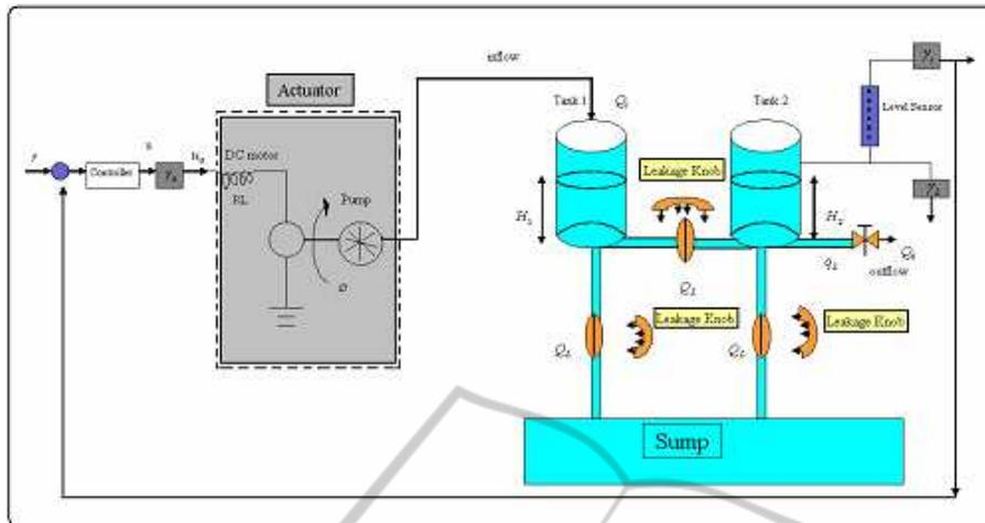
Figure 2: Two tank model.
