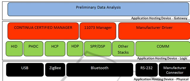
Fig. 2. Application Hosting Device Stack.
