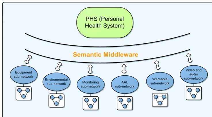
**Fig. 1.** Proposed Architecture for a Personal health System. Sensors are grouped into sub-networks, where an Application Hosting Device (AHD) acts as a data concentrator and intelligent gateway towards the Semantic Middleware.
