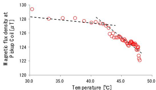
Figure 7: Relationship between temperature of FILCT and the voltage of the pickup coil.
