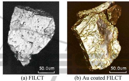
Figure 2: Micrograph of a particle of the ferromagnetic implant with low Curie temperature.
