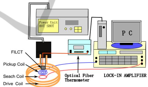
Figure 3: Block diagram of the experimental setup of the less-invasive heating and thermometry.
