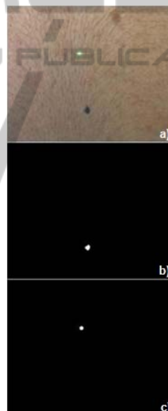
Figure 7: Aspect of the blue and green laser mark on the skin (a); Binarization plus opening operation of the blue mark (b); Binarization of the laser mark (c).
