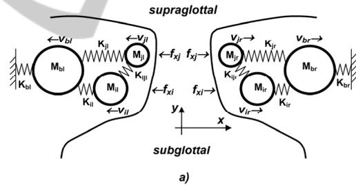
Figure 4: Vocal Fold Biomechanical Model of Story and Titze (see text for details).
