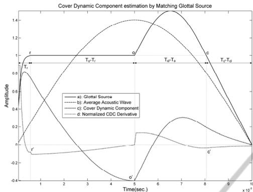
Figure 2: The LF Glottal Cycle. Top: In full black line the GS Ideal pattern. Bottom: Real pattern obtained from a prototype male speaker (normophonic).
