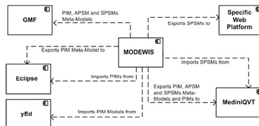
Figure 6: The Architecture of MODEWIS.
