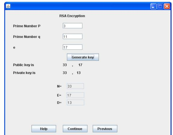
Figure 6: Use RSA to generate keys.
