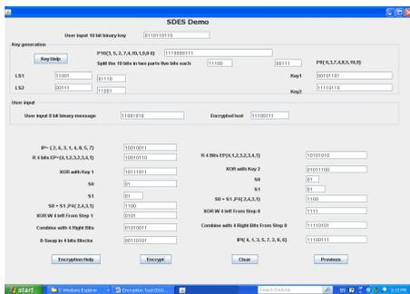
Figure 4: A demonstration of using SDES.
