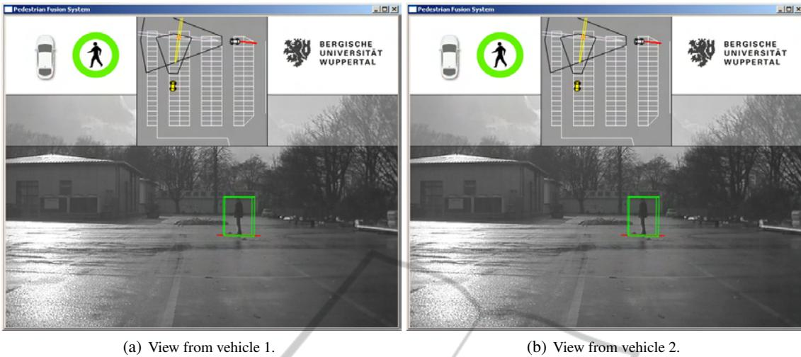
Figure 4: Results of pedestrian detection fusion from two vehicles. Fig. 4(a) and 4(b) are recorded at the same timestamp. The ego vehicle is gray and the remote vehicle is yellow. The trajectory of the vehicles is denoted by red dots.
