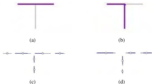
Figure 4: 2D example for different linking of the T-shape. (a) & (b) Show differently linked edges that form longer contour fragments, (c) & (d) represented as GMMs.
