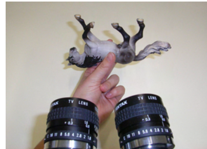
Figure 7: Stereo rig to capture the database. We use two \mu Eye 1220C cameras and Cosmocar/Pentax lenses with a focal length of 12.5 mm. The baseline is approximately 6cm (human eye distance), the vergence angle 5.5^\circ . The frame rate is 15 Hz. The size of the images is 480x752 px. For the calibration of the stereo rig we use the Camera Calibration Toolbox for Matlab (Bouguet).
