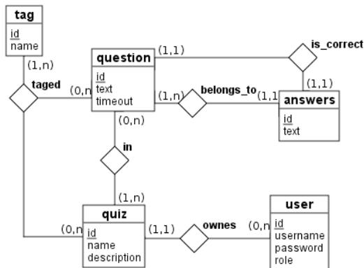
Figure 2: ER diagram of database.
