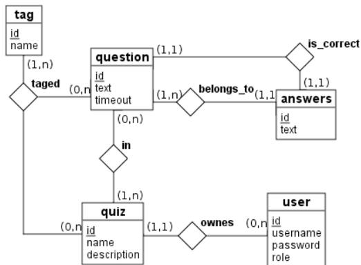
Figure 2: ER diagram of database.
