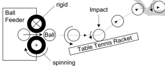
Figure 1: Data acquisition setting.
