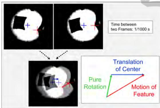
Figure 4: Calculating rotational displacement.
