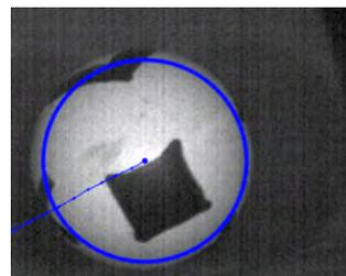
Figure 3: Circle fitting to ball contour.
