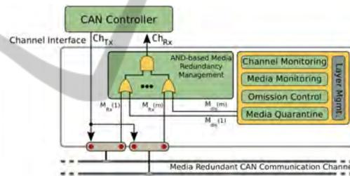
Figure 6: CANELy Media Redundancy Mechanisms.
