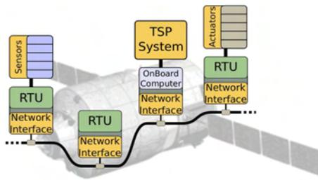
Figure 1: Utilization of CAN in a spacecraft TSP system.
