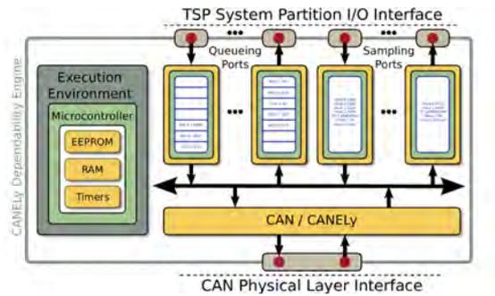
Figure 13: CANELy Dependability Engine extension with support for distributed TSP systems.
