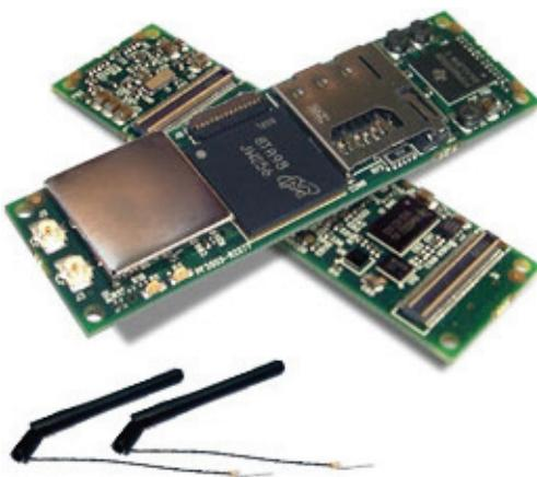
Figure 2: The Single Board Computer System.
