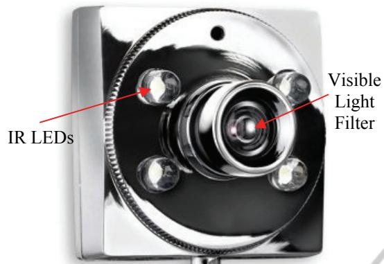
Figure 4: The modified camera.
