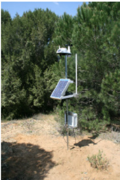
Figure 6: Example of an anchor node.
