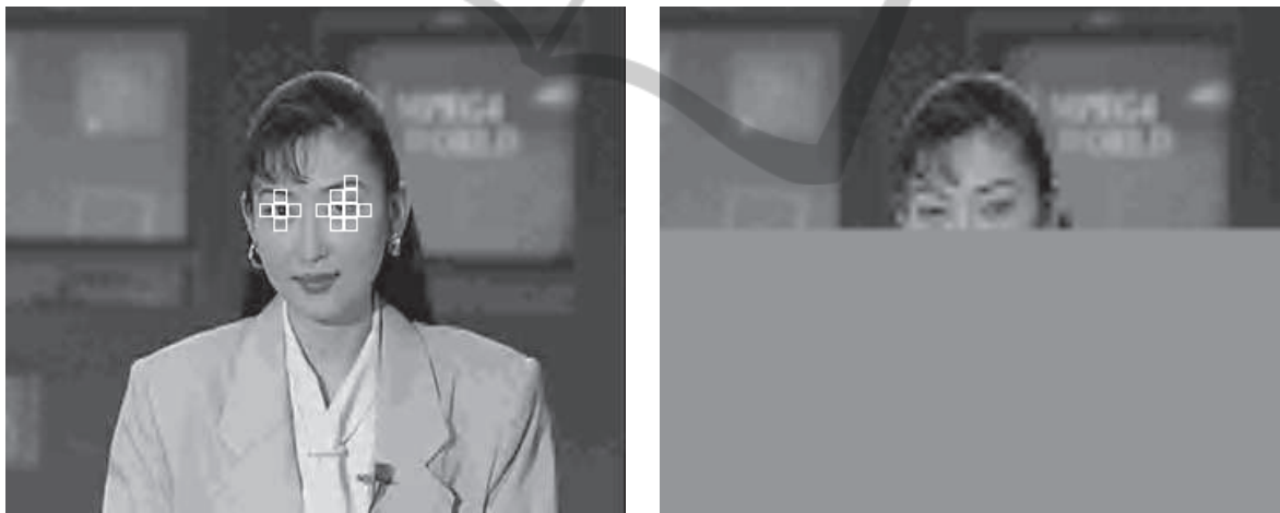
Figure 5: Two Akiyo reconstructed images, left with and right without CR. The refreshed precincts have been highlighted with a white square.
