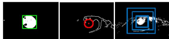
Figure 7 Binarized image of the pupil (left); Edge and circle detection (middle); Sequential Mean-shift (right).
