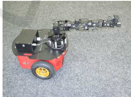
Figure 1: Pioneer 3DX mobile robot with manipular.
