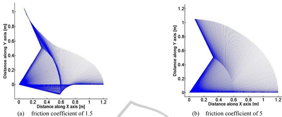
Figure 5: Results for the designed optimal path in terms of temporal positions for increasing friction values.
