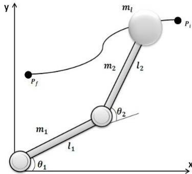
Figure 2: Schematic diagram of the robot and a prescribed trajectory given by initial and final points.
