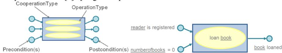
Fig. 5. Graphical notation of a CooperationType and Example.
