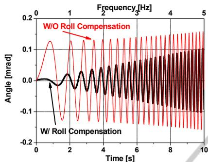
Figure 4: Stabilization error – azimuth direction.
