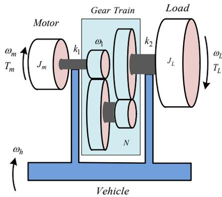
Figure 2: Schematic of gimbal driving mechanism.
