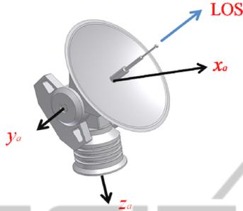
Figure 1: Structure of OTM Antenna.
