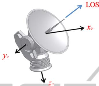
Figure 1: Structure of OTM Antenna.
