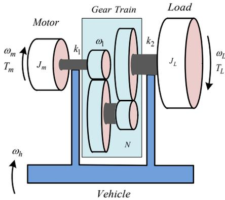
Figure 2: Schematic of gimbal driving mechanism.
