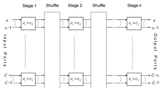
Figure 1: The general structure of a delta network.
