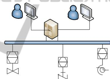
Figure 2: A typical Networked SCADA System.
