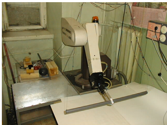
Figure 1: Robot Manipulator PUMA 560. Grasping the Rod on Bifilar Suspension.
