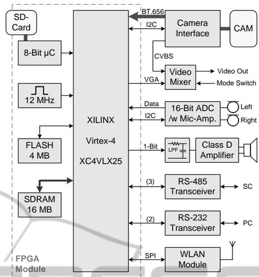
Figure 4: On the one hand the BRAINMODULE is just another processing node of the DISTAL architecture, but on the other hand it possesses considerably more processing power than an ACCELBOARD3D. This is needed for the audio-visual processing inside the robot's head.
