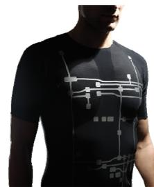
Figure 1: Vital Jacket, the wearable very long-term ECG recording device used in the study.
