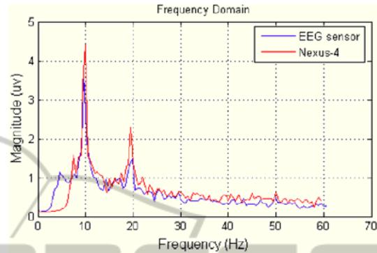
Figure 16: Frequency Response Comparison with NEXUS-4.
