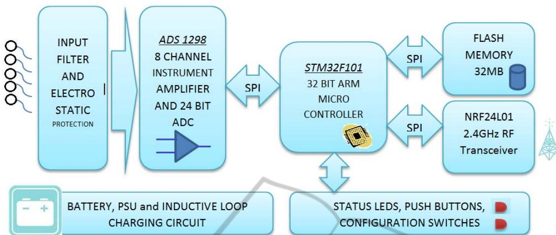
Figure 1: EEG Sensor, primary hardware components.
