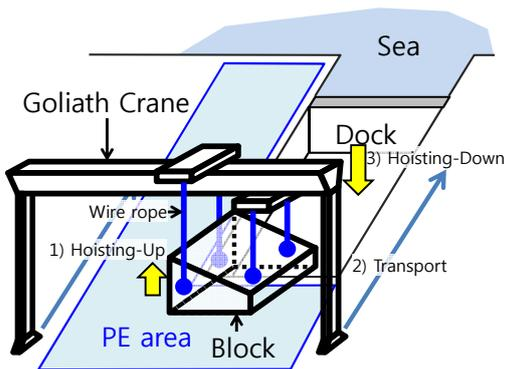
Figure 6: Block-lifting and transport process.
