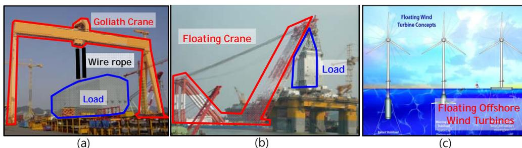
Figure 1: Various types of mechanical systems in the shipbuilding industry: (a) goliath crane; (b) floating crane; and (c) floating offshore wind turbines.
