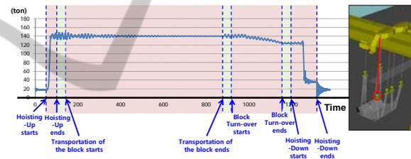
Figure 10: Tension of the wire rope, which is marked with red, calculated by using developed program.
