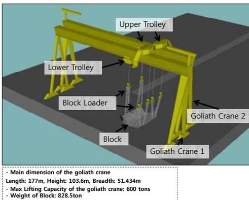
Figure 9: The goliath cranes and block model in the simulation of the block-lifting and transport.
