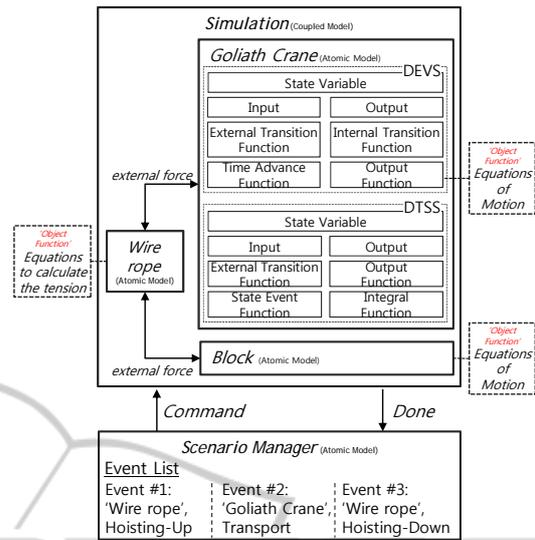
Figure 7: DEVS simulation model for the block-lifting and transport simulation.
