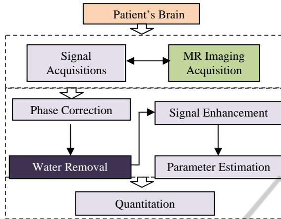
Figure 1: Block diagram for <sup>1</sup>H MR spectroscopy analysis.
