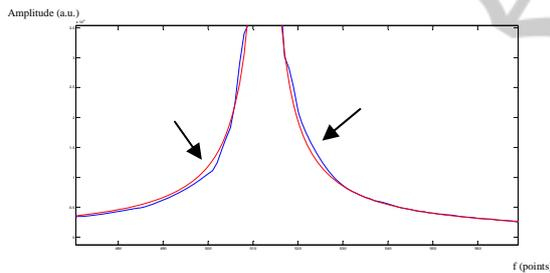
Figure 3: Imperfect reconstruction of water contribution to subtract it from the original signal. In blue and in red the original and the reconstructed signal respectively.
